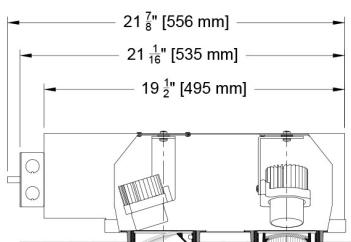
NOTE: This option is intended for use with precise and finished cutouts - usually millwork or wood ceilings. There is no plaster or finish flange.
